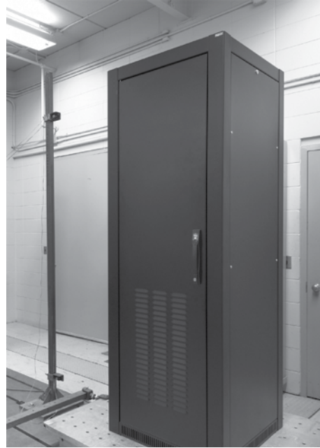
Enclosure mounted on shaker table
